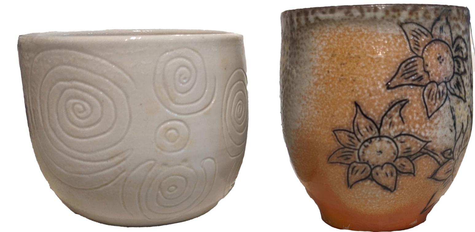
Oxidized soda-fired porcelain (L) Reduced soda-fired porcelain (R)
